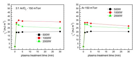
Fig. 1. The polar  $\gamma_s^p$  component of the free surface energy of PC treated in Ar and 3:1 Ar/O<sub>2</sub> plasma vs treatment time at indicated RF power.
